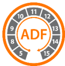
Zakres zaciemnienia filtra ADF (SA60 = 5-13, XA74 = 5-15)
